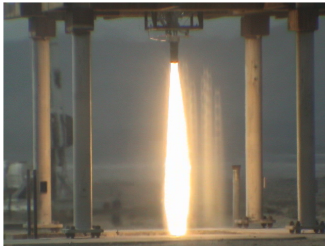
Figure 2. CALVEIN LOX/Propylene Engine Static Fire Test 11/2004 iii
