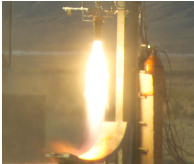
Figure 2. LOX/Propylene Engine Static Fire Test 11/2008
